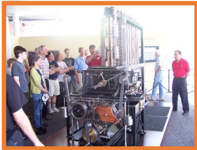
1832, 2002, 2008 The Babbage Difference Engine, 17 years, 25,000 parts, 5ton, cost: £17,470
